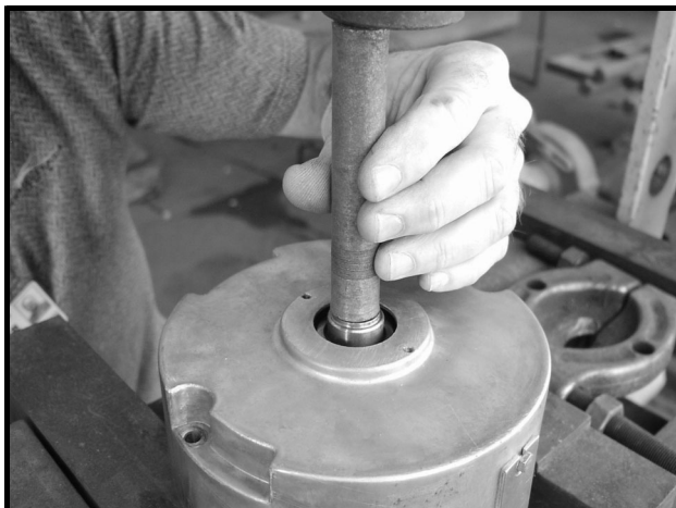
Figure 16b-8 Armature Removal
