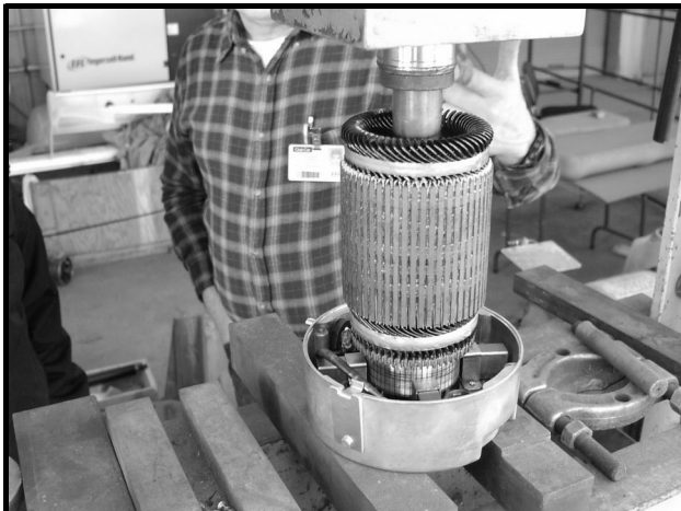
Figure 16b-18 Armature Installation
